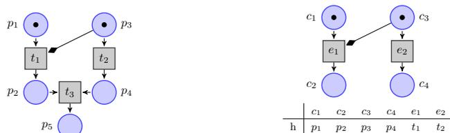
■ **Figure 1** A reset Petri net (left) and one of its processes (right)
