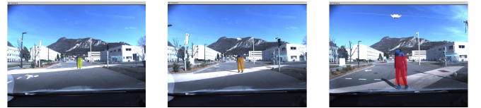
Fig. 8. Risk detection combined with automatic braking sequence. The evolution of the color of the reprojected collision risk corresponds to the time window before impact, activating accordingly the automatic braking.
