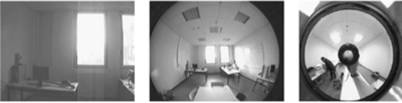
Figure 1. Three images acquired approximately at the same position, with a 1/4-inch image sensor with a perspective lens (left), the same image sensor with an Omnitech Robotics ORIFL190-3 fisheye lens with a field of view of 190^\circ (middle) and a catadioptric camera (right).
