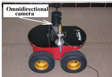
Fig. 15 Mobile robot Pioneer 3 equipped with an omnidirectional camera
