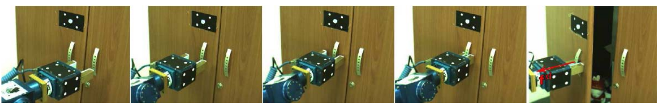
Fig. 4. Reaching the handle. (a) Initial position (b) Reaching the pre-grasp position (c) Reaching the grasp position (d) Grasping (e) Interaction.
