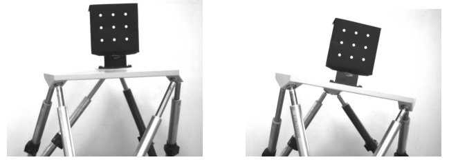
Fig. 3. Initial (left) and desired (right) position of the end-effector, seen from the camera.
