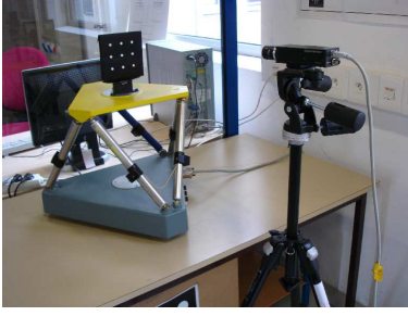
Fig. 1. A Gough-Stewart platform observed by a camera.
