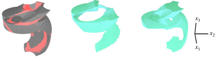
Figure 6: Computed 3D workspace of 3-RPR (after filtering). First figure shows the undecided boxes that cover the surface of the workspace. Second and third figures show the computed CSNCs corresponding to the two aspects.
