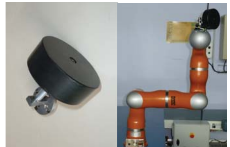
Fig. 2. The payload of 4.6136kg for the Kuka LWR.
