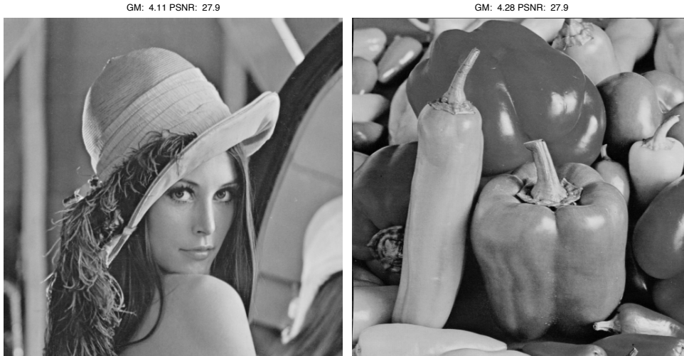
Figure 7: “Lena” and “peppers” after the same geometrical distortion. The left image is visibly corrupted (look at the vertical structure on the left), while the right one looks perfect. The PSNR is not able to catch the perceptual quality difference of these images, while the GM is, as shown in Table 1
