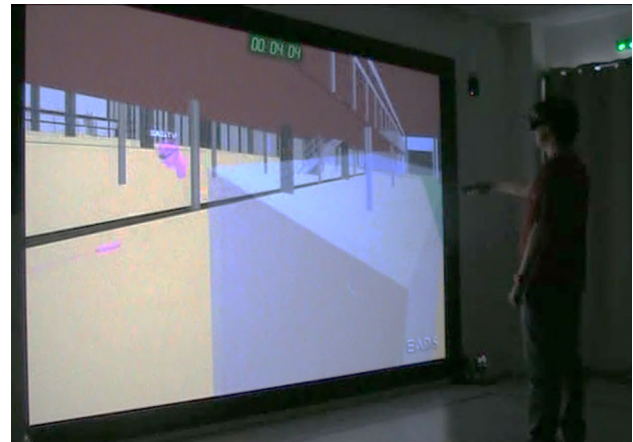
Fig. 1 Picture of a participant in front of the immersive wall. The pink head with the black glasses on the left of the picture is the avatar of the remote collaborator. The transparent blue cuboid on the right of the screen is the object the manipulator participant had to move in the virtual environment (color figure online)
