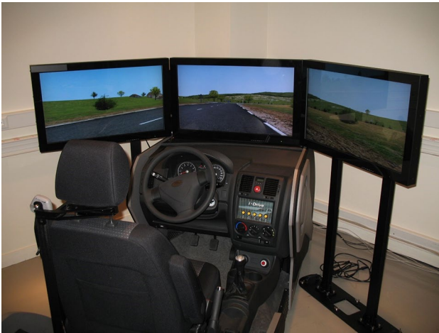
Fig. 2 The fixed-base driving simulator
