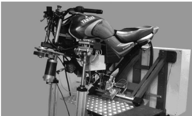
Figure 1. Motion-based motorcycle simulator.
