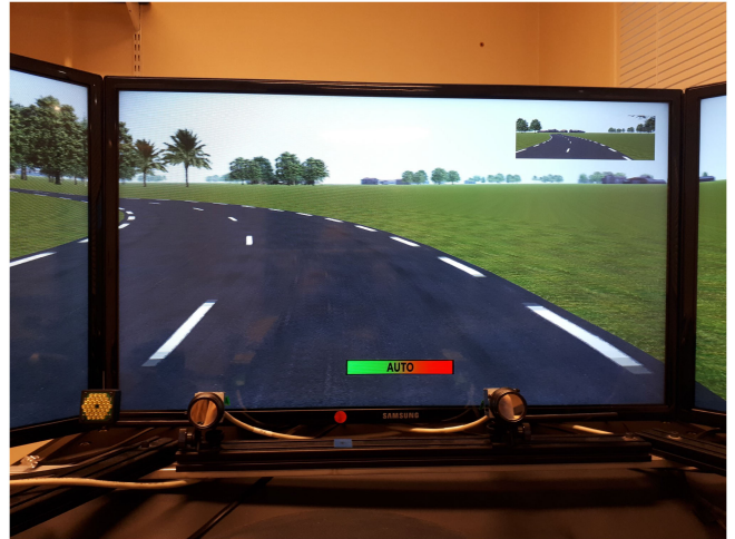
Fig. 4. Center screen of the simulator displaying the progressive bar while in autonomous mode.
