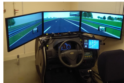
Figure 1. Driving simulator setup
