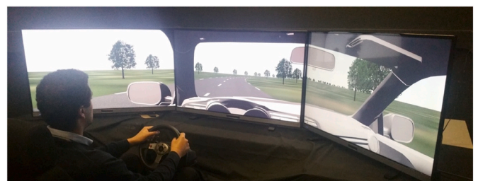
Fig. 1. Illustration of the low-cost driving simulator with a virtual full-scale cab displayed in the visual scene.
