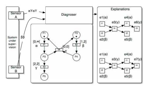
Fig. 1. Model-based diagnosis of distributed systems using time Petri nets.
