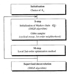
Fig. 2. Schematic representation of the unsupervised deconvolution procedure.
