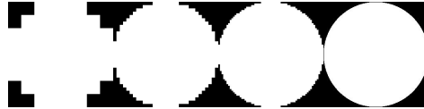
Fig. 12. Pupil shape in the PD algorithm for three numbers of pixel used in the pupil sampling [8, 32, 64 and 256]. The oversampling factor of 2 in K band leads to corresponding image sizes equal to [32, 128, 256 and 1024].
