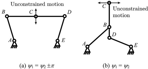
Fig. 2 Type 2 singular configurations of the planar 5R parallel manipulator
