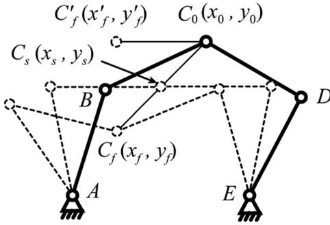
**Fig. 3 Initial, singular and final positions of the planar 5R parallel manipulator**
