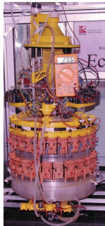
Ecobot 3: was capable of operating within an enclosed environment for 7 days, by collecting its food and water from the arena environment (2010)
