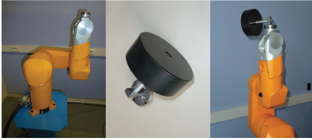
Fig. 1 TX-40 robot and its calibrated payload of 4.59 kg
