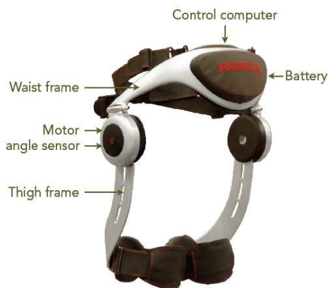
Figure 19. Walking assist device with stride management assist.
