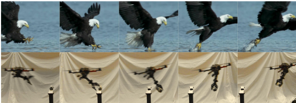
Fig. 1.2. A still image comparison between the eagle and the quadrotor for a trajectory with the quadrotor moving at 3 m/s (9 body lengths/s) at pickup.[35]
