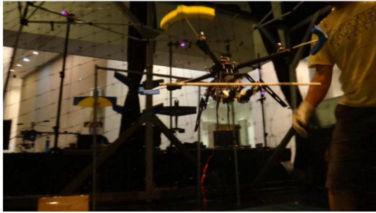
Fig. 1.4. MM-UAV carrying a long rod[20]
