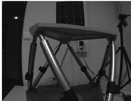
Figure 2.4: Left: a Gough-Stewart platform from DeltaLab; Right: schematics of leg i
