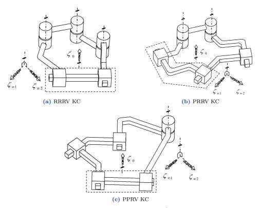
**Figure II.3** – Single-loop Kinematic Chain 2 *dof*,  $c^i = 3$  (Perpendicular Case)
