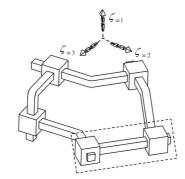
**Figure II.5** – Single-loop Kinematic Chain 2 dof,  $c^i = 3$ : PPPV KC
