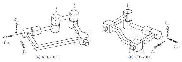
**Figure III.3** – Single-loop Kinematic Chain  $c^i = 3$
