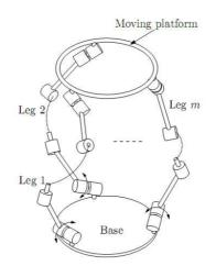
Figure I.1 – Parallel Kinematic Chain [17]
