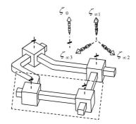
**Figure II.2** – Single-loop Kinematic Chain 2 *dof*,  $c^i = 4$ : PPV KC
