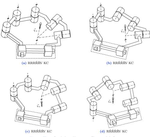
**Figure II.9** – Single-loop Kinematic Chain 2 dof,  $c^i = 1$
