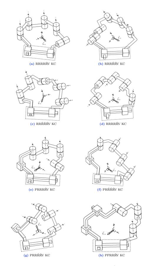
**Figure II.8** – Single-loop Kinematic Chain 2  $\mathit{dof},\, c^i=1$
