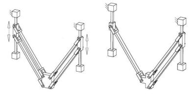
Figure I.7 – 2 dof PM for Machine Tool [18]
