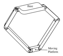
**Figure V.4** –  $\underline{R}RR-U\underline{R}U$  Parallel Manipulator
