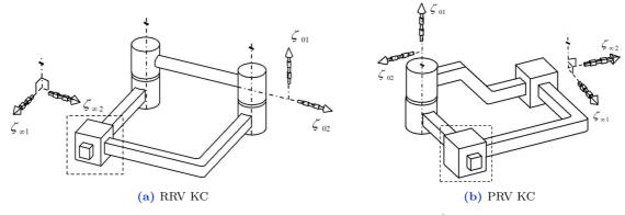
**Figure III.2** – Single-loop Kinematic Chain  $c^i = 4$
