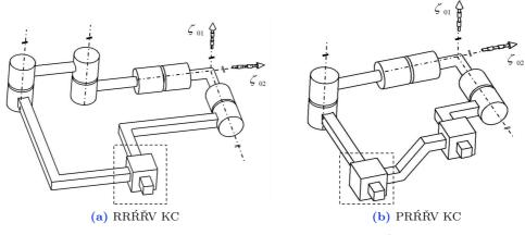
**Figure III.4** – Single-loop Kinematic Chain  $c^i = 2$
