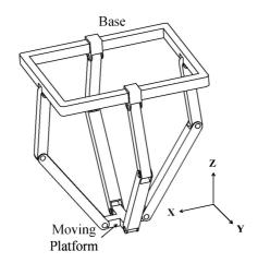
Figure V.2 –  $2-\underline{R}RR-2-PRRR$  Parallel Manipulator
