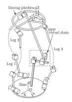
**Figure I.13** – 3 *dof* PM with Virtual Chain [17]
