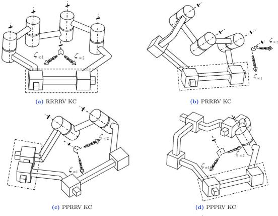
**Figure II.7** – Single-loop Kinematic Chain 2  $dof, c^i = 2$
