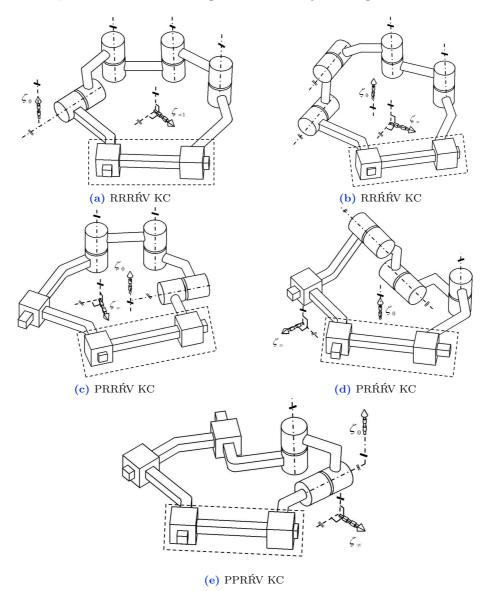
**Figure II.6** – Single-loop Kinematic Chain 2 dof,  $c^i = 2$
