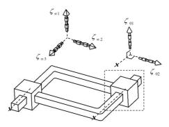
**Figure III.1** – Single-loop Kinematic Chain  $c^i = 5$ : PV KC
