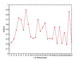
**Figure V.8** – Stiffness Index with Bending Forces and Moments
