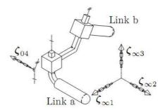
Figure I.11 – Twist and Wrench System of PP Serial Kinematic Chain [17]
