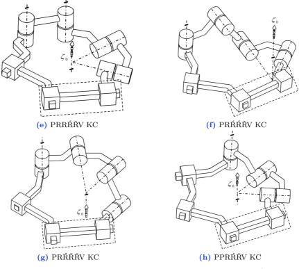
**Figure II.9** – (Continued) Single-loop Kinematic Chain 2 dof,  $c^i = 1$
