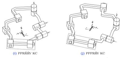
**Figure II.8** – (Continued) Single-loop Kinematic Chain 2  $dof, c^i = 1$
