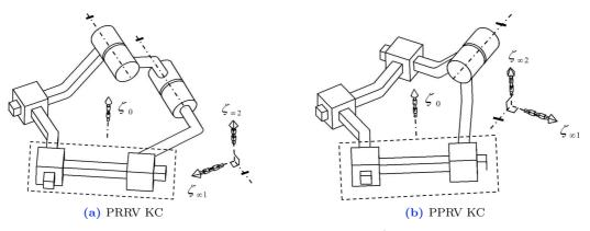
**Figure II.4** – Single-loop Kinematic Chain 2 dof,  $c^i = 3$  (General Case)
