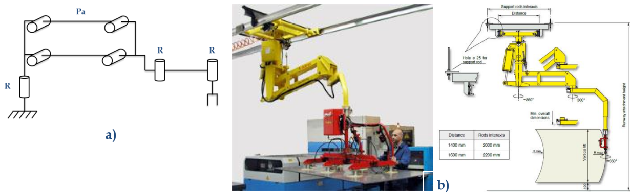
Figure 2.4 (a) Kinematic structure of an RPaR-R orthogonal manipulator (b) RPaR orthogonal DALMEC Maxipartner MXS manipulator (from [16])
